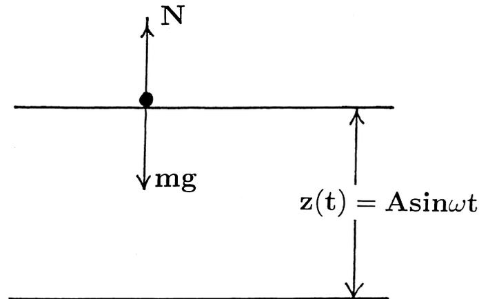
Fig. 2. Particles of mass  $m$  initially resting on a horizontal plate which is moving according to  $z(t) = A \sin \omega t$ .
