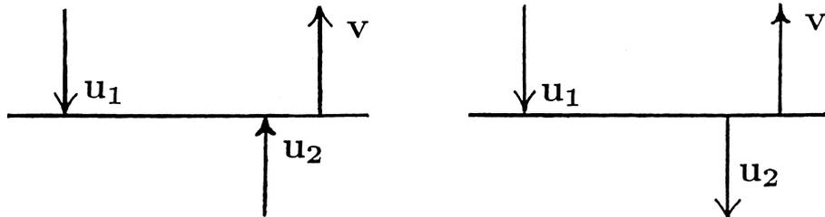
Fig. 3. Falling particles impacting on both upwards and downwards moving plate, arrows indicating direction of movement: (a) plate moving upwards; (b) plate moving downwards and  $u_1 > u_2$ .
